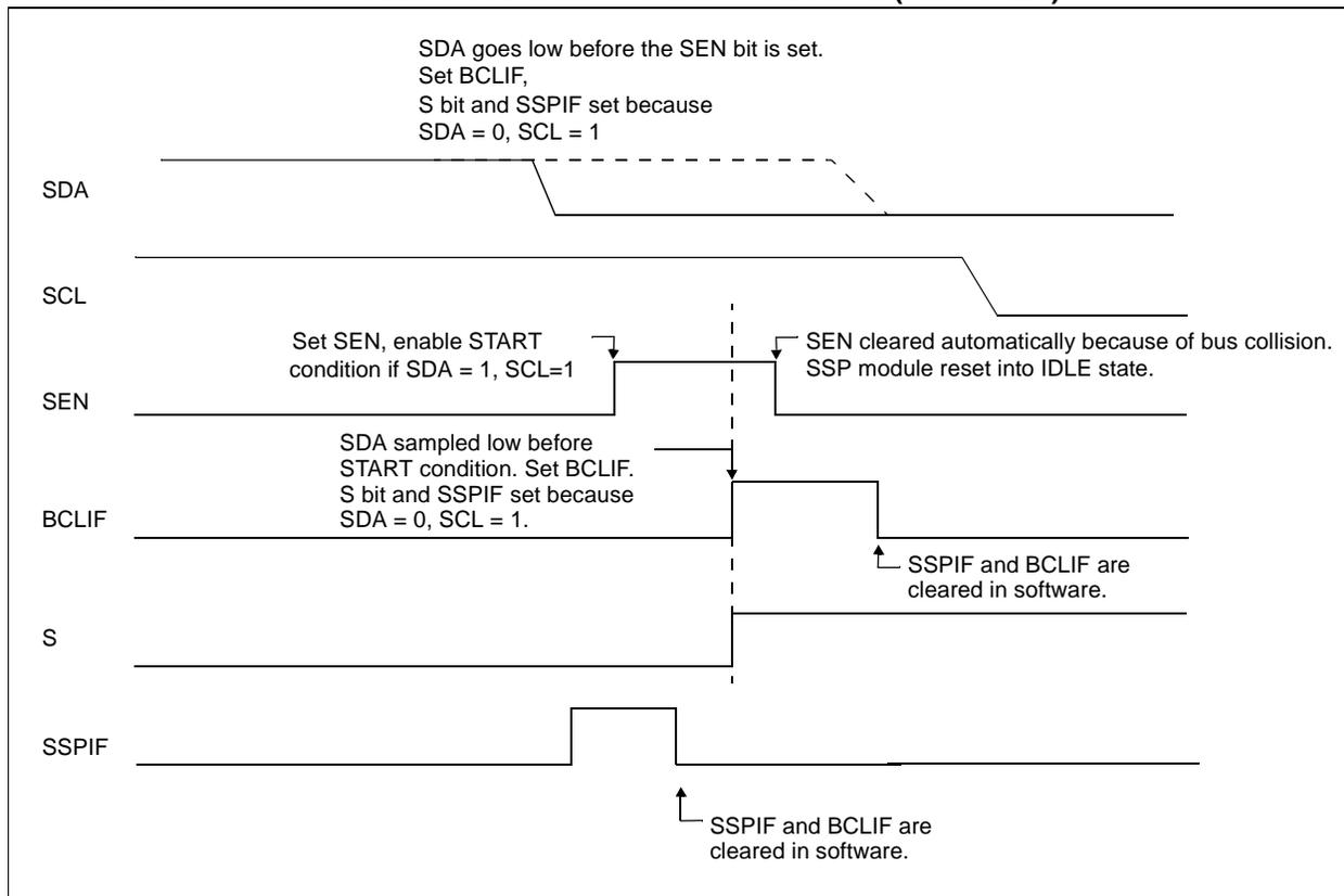
**FIGURE 9-27: BUS COLLISION DURING START CONDITION (SCL = 0)**
