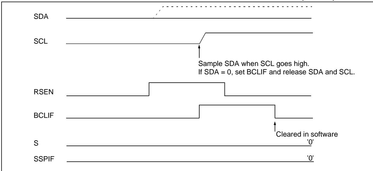
**FIGURE 9-30: BUS COLLISION DURING REPEATED START CONDITION (CASE 2)**
