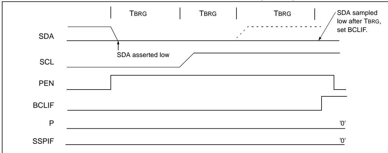
**FIGURE 9-32: BUS COLLISION DURING A STOP CONDITION (CASE 2)**
