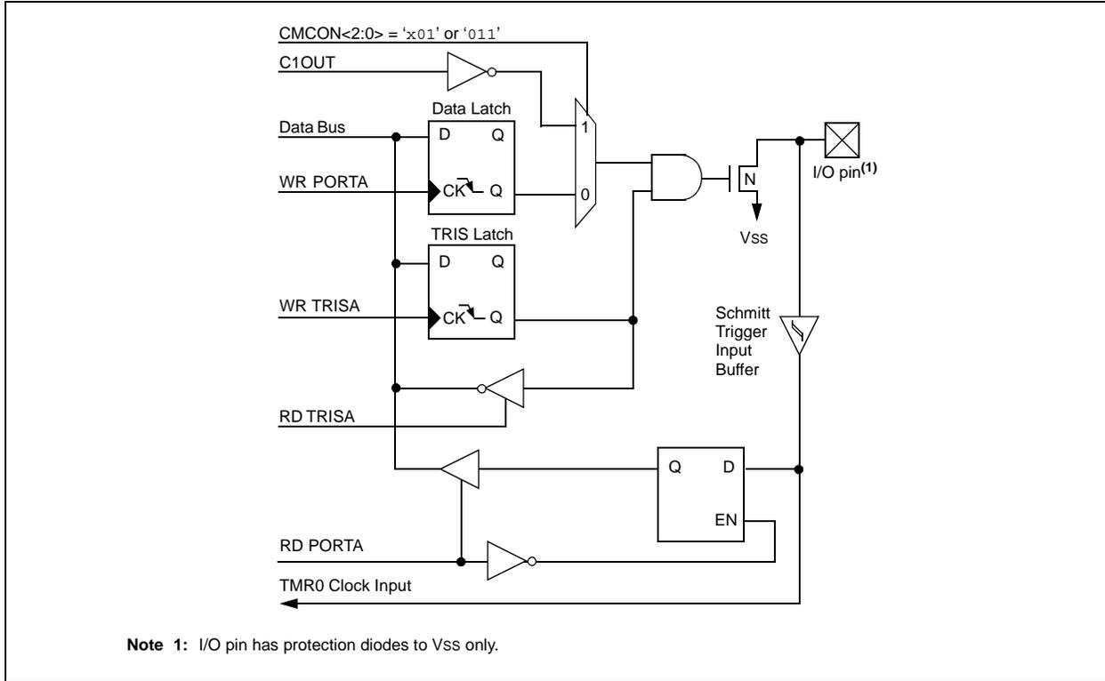
**FIGURE 4-3: BLOCK DIAGRAM OF RA5 PIN**
