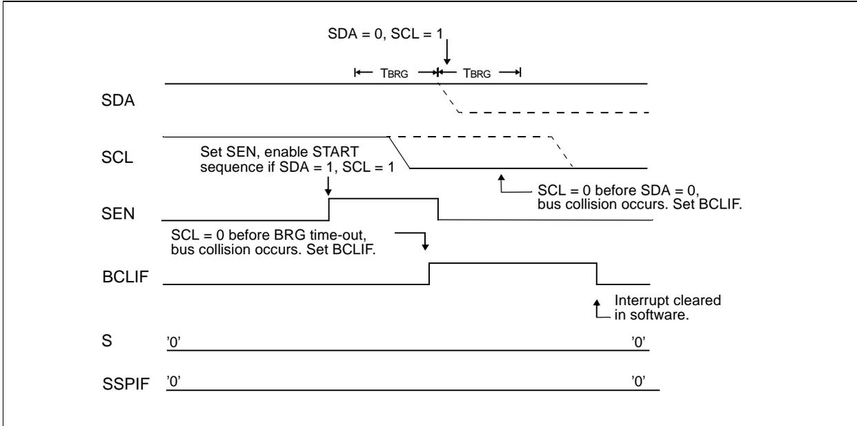
**FIGURE 9-28: BRG RESET DUE TO SDA ARBITRATION DURING START CONDITION**
