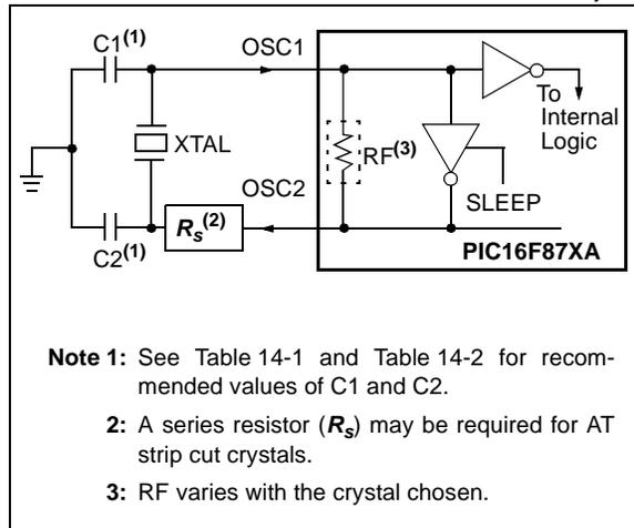
**FIGURE 14-2: EXTERNAL CLOCK INPUT OPERATION (HS, XT OR LP OSC CONFIGURATION)**
