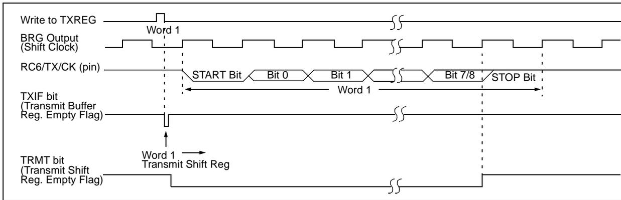
**FIGURE 10-3: ASYNCHRONOUS MASTER TRANSMISSION (BACK TO BACK)**
