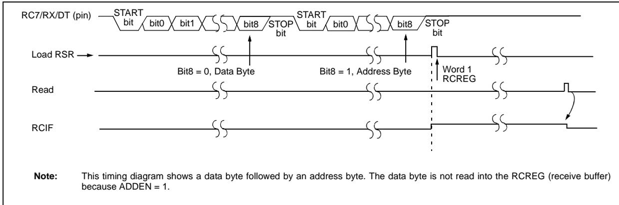
**FIGURE 10-8: ASYNCHRONOUS RECEPTION WITH ADDRESS BYTE FIRST**
