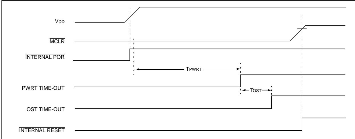
**FIGURE 14-9: SLOW RISE TIME ( $\overline{\text{MCLR}}$  TIED TO  $V_{DD}$  VIA RC NETWORK)**
