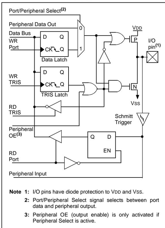
**FIGURE 4-7: PORTC BLOCK DIAGRAM (PERIPHERAL OUTPUT OVERRIDE) RC<4:3>**
