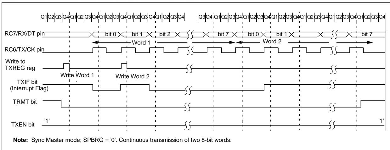
**FIGURE 10-10: SYNCHRONOUS TRANSMISSION (THROUGH TXEN)**
