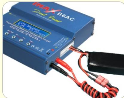
The main battery leads must be connected along with the balance lead connector as shown before charging your battery ..
