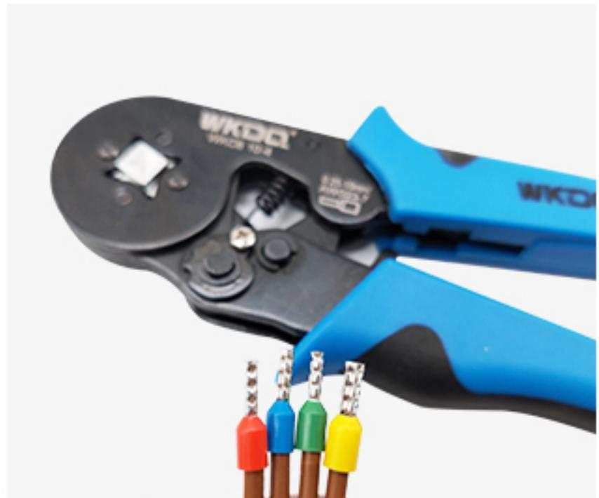
4. Take out the ferrule, and make the tension testing.
