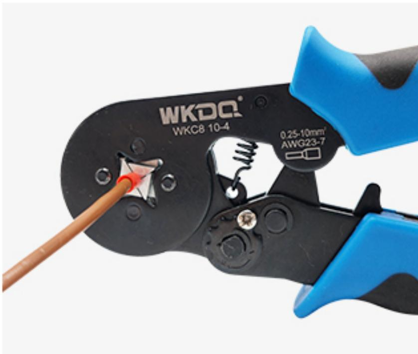
3. Put the ferrule into the crimping hole, and press the handle, after hear a click sound, then release the handle.
