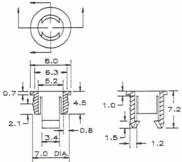
**PT18H013** is a black PP mounting clip and retain ring. It is designed to panel mount Ledtech part number UT18XX-XX lamps. This clip and ring combination is intended for installation instrument panels from 0.5mm to 2.7mm. For panels greater than 2.7mm counterboring is required to the 2.7mm thickness. The acceptable hole diameter in the panel will be 6.3mm.
