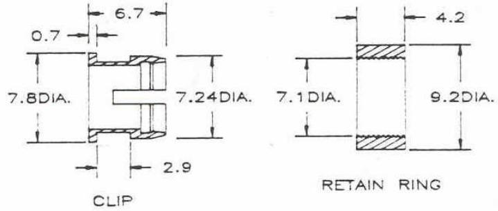
**PT03H010** is a black PP mounting clip. It is designed to panel mount Ledtech part number UT03XX-XX lamps. This clip is intended for installation instrument panels of 1.6mm thickness. The acceptable hole diameter in the panel will be 4.6mm.
