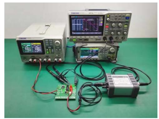
SDS1000X-E can control the USB AWG module or control an independent SIGLENT SDG instrument, scan a device's amplitude and phase frequency response, and display the data as a Bode Plot. There is also a Vari-level Mode for accurately measuring Power Supply Control Loop Response (PSRR). It can also show the result lists, and export the data to a USB disk.
