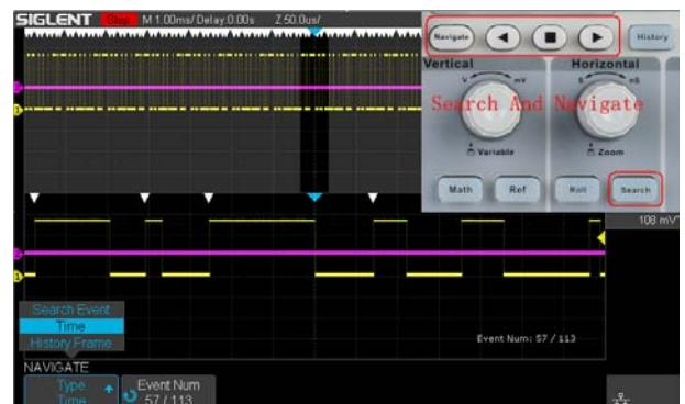
The SDS1000X-E can search events specified by the user in a frame. It can also navigate by time (delay position) and historical frames.
