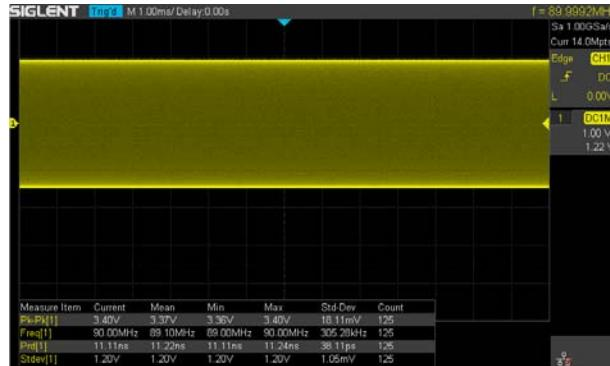
SDS1004X-E can measure all sampled data points up to 14 Mpts. This ensures the accuracy of measurements while the math co-processor decreases measurement time and increases ease-of-use.
