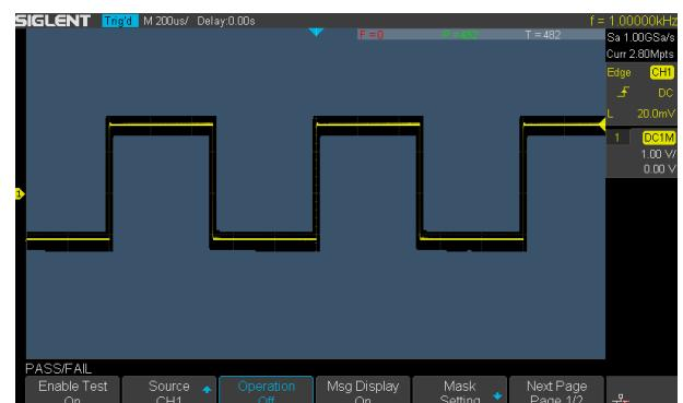
The SDS1000X-E utilizes a hardware-based Pass/Fail function, performing up to 40,000 Pass / Fail decisions each second. Easily generate user defined test templates provide trace mask comparison making it suitable for long-term signal monitoring or automated production line testing.
