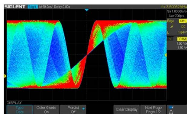
The color temperature display is similar to the intensity-graded trace function, but the trace occurrence is represented by different colors (color "temperature") as opposed to changes in the intensity of one color. Red colors represents the more frequent events, while blue is used to mark points that occur least frequently.
