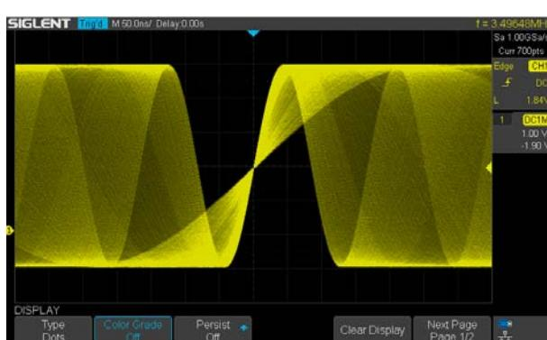
SPO display technology provides fast refresh rates. The resulting intensity-graded trace is brighter for events that occur with more frequency and dims when the events occur with less frequency.
