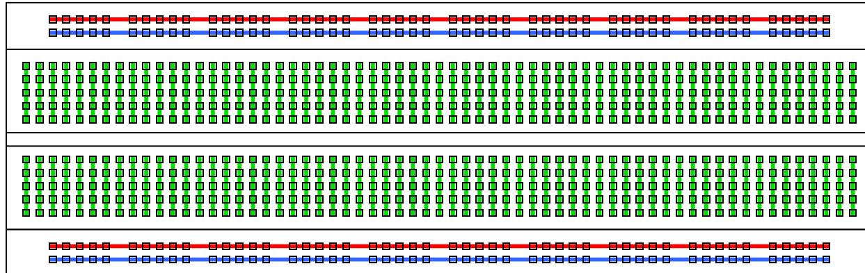
The BB830 and BB830T breadboards have 63 vertical columns on top and 63 columns below. Each column has 5 connected holes each (the green lines). This is the circuit area. There are also 4 "rails" (or distribution strips) for power and ground running horizontally (the red and blue lines). A distribution strip can be used to carry a signal if it is not needed for power or ground.
