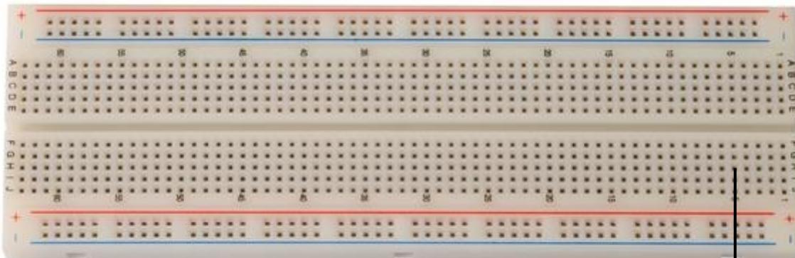
**BB830** - 830 tie-point plug-in Solderless BreadBoard, ABS plastic with color legend
