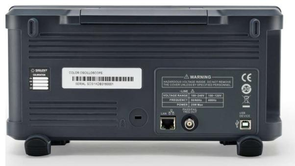
SDS1000X-E supports USB Host, USB Device (USB-TMC), LAN (VXI-11), Pass/Fail and Trigger Out
