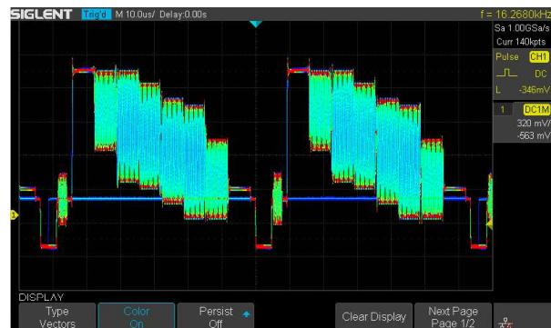
The color temperature display is similar to the intensity-graded trace in function, except that the trace occurrence is represented by different colors (color "temperature") as opposed to changes in the intensity of one color. Red represents the most common occurrences or probabilities, while blue is used to mark points that occur least frequently.
