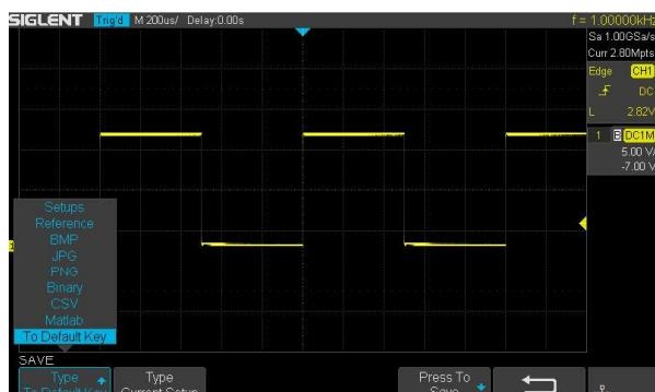
The current parameters of oscilloscope can be preset to Default Key through the Save menu.
