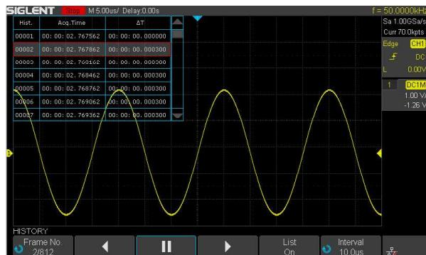
Playback the latest triggered events using the history function. Segmented memory acquisition will store the waveform into multiple (up to 80,000) memory segments, each segment will store triggered waveforms and timestamp each frame.
