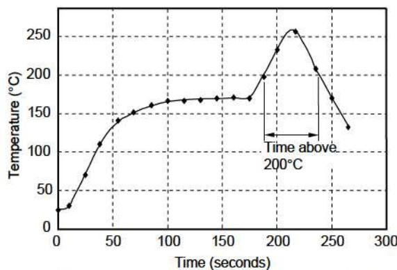
The times of repeated reflow soldering must be two times or less.
