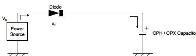
You do not need to insert a resistor to regulate charging current.
