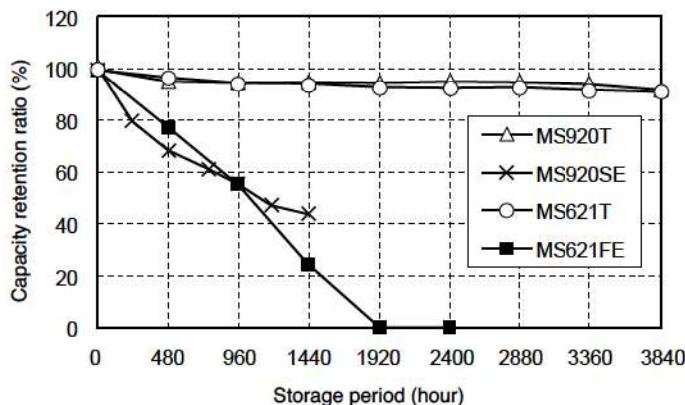
MS-T series's capacity retention ratio after High temperature storage were greatly improved.
