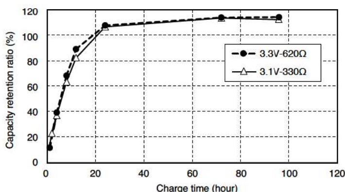
Both the MS621T and MS920T can reach 80% of capacity after 12 hours of charging.
