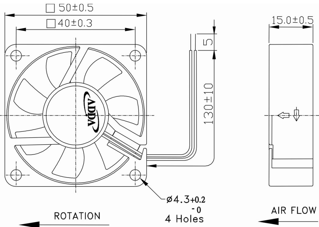
LEAD WIRES : UL 1007, AWG26 , L = 130 +/- 10 mm
