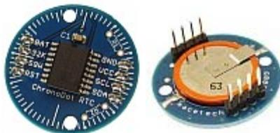
The [ChronoDot RTC](#) is an extremely accurate real time clock module, based on the DS3231 temperature compensated RTC (TCXO). It includes a CR2016 battery which should last at least 8 years if the I2C interface is only used while the device has 5V power available. No external crystal or tuning capacitors are required.
