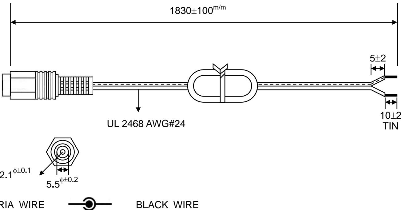
FUNCTION TEST: No open, no reversed polarity, no short-circuit, no INT
