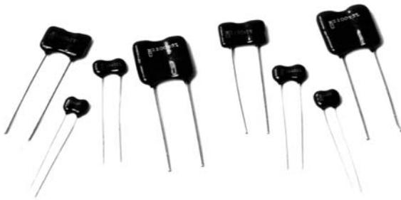
Nearly the textbook ideal capacitor for high-frequency applications, Type CD4 is rock stable over its full temperature and voltage range. Higher self-resonant frequency and lower equivalent series inductance makes CD4 even better than CD17 and CD18 for high-frequency applications. 0.1" lead spacing means CD4 can replace ceramic capacitors on printed circuit boards.
